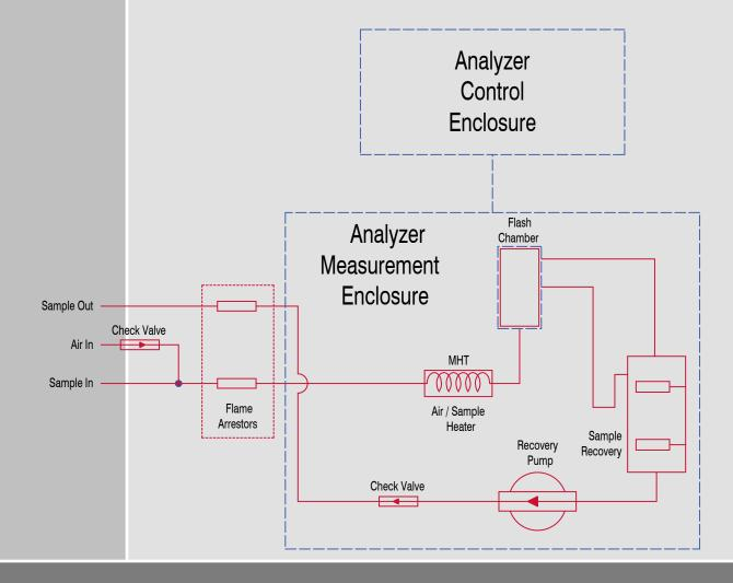
First, the sample and combustion air are externally mixed. This mixture then enters the lower analyzer enclosure. This mixture then enters the sample mixing and heating tube (MHT). The specially designed MHT allows for uniform mixing of combustion air and then the controlled heating of the continually flowing sample.
